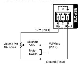
Figure 5. Remote Control Wiring
